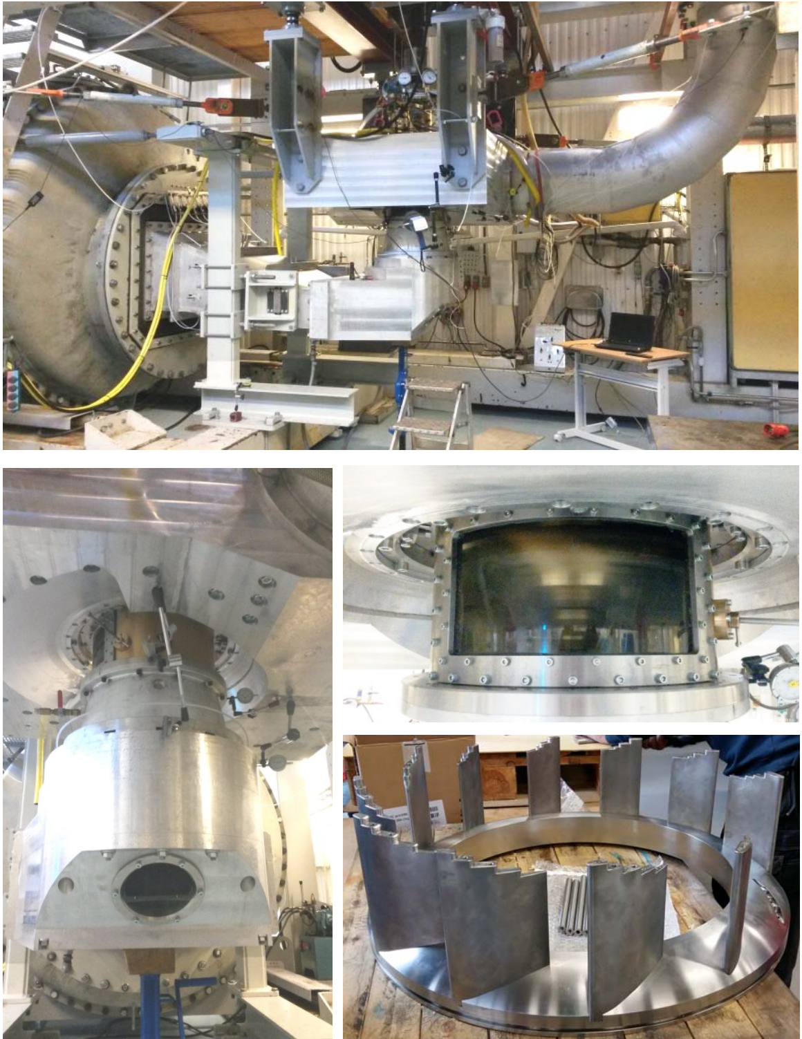
Figure 3.3 An example of a Kaplan model turbine installed in Vattenfall test rig.
